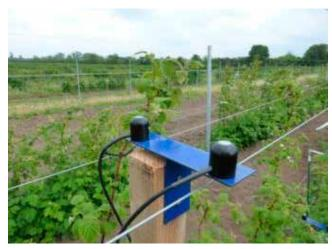
Figure 3: PYR Apogee SP-110 360-1120 [nm] and PAR Apogee SQ-100 380-720 [nm]
