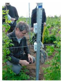
Figure 4: Temperature sensors at: - 0,15 [m], 0 [m], 1,0 [m], 1,8 [m].
