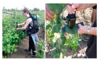
Figure 6: ASD FieldSpec 3 MAX with PlanProbe sensor head and a Cubert snapshot camera
